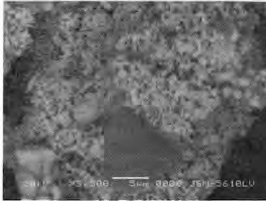
Fig 2(a): Ag-3%C as-blended powder showing heterogeneously dispersed grey coloured graphite particles in silver matrix
