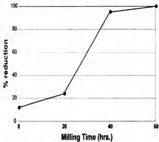
Fig.3 Percent reduction of mill scale as a function of the milling time.
