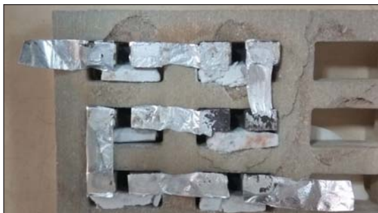
Fig.8 : TEG circuit made from unicouples (p and n type legs)
