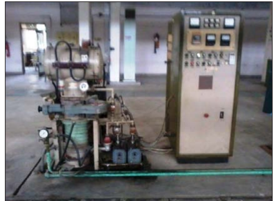
Fig. 3 : Electric Resistance Batch-type Vacuum Furnace (Courtesy ARCL, Hyderabad)
