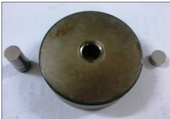
Fig. 1: Die and punch set to fabricate cylindrical preform
