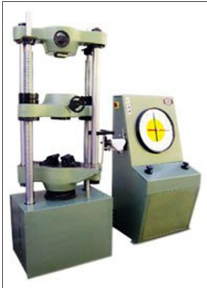
Fig. 2 : Universal Testing Machine for preparing the green compacts (Courtesy ARCL, Hyderabad)
