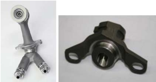
Fig.7: Some PM components manufactured by AM technique
