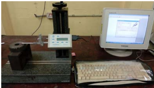
Fig. 5 : Taylor Hobson Surface Roughness Tester at Metrology Lab, JU
