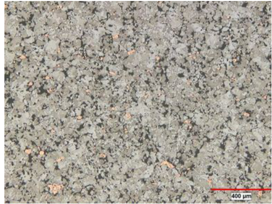
Fig. 2: Photomicrograph showing the distribution of -15 micron copper particles in FC-0208
