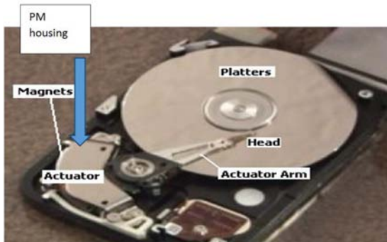
Fig. 5: Disk drive with PM housing and NdFeB magnets, ref 12
