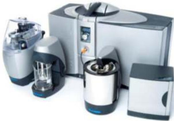
The Mastersizer 3000 can analyse powders in dry form or suspensions/slurries of the same. The dry powder dispersion unit Aero S can control dispersive air pressure very precisely. The following histogram indicates that there is no impact of dispersive air pressure on the sample AlSiO<sub>2</sub>.
